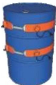
Marathon Heater Drum Heaters are an easy way to heat up drum contents. Various sizes and lengths allow you to heat up practically any drum, pail or barrel. Uniform heat prevents scorching or degradation of the contents. The silicone rubber band heater is placed below the level of the fluid. The easy spring lock-up provides movement of the band when content levels fluctuate. The band style drum heater can be used on plastic, alloy or just about any material.
